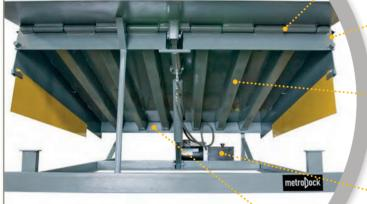
3. High Tensile **Formed "A" Beam**, a standard on docks up to 35,000 lbs. capacity. Wide flange I-beam construction on capacities 40,000 lbs. up to 100,000 lbs.
