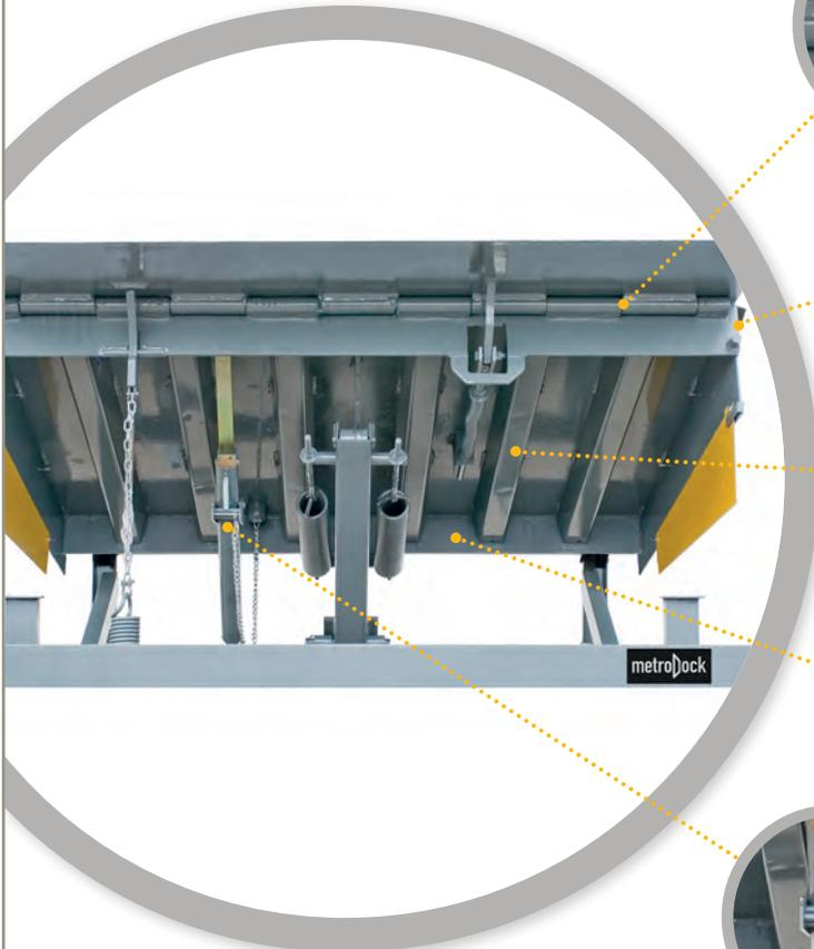
1. **Lip Hinge & Pin** – Constructed of high tensile continuous seamless tube (minimum 70,000 lbs. yield) and a one piece hinge pin, provides superior strength and enhanced durability.
