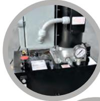
1. Remote **Powerpack** standard 5-HP North American made c/w self-contained adjusting valves.
